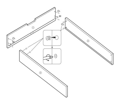
Use the wooden connectors (Part M) and bolts (Part O) to combine the side (Part 2) with the front board of the drawers (Part 1).
