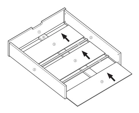
As the illustrated direction, slide the parts (Part 3 & 4) into the assembled parts in step 2.
