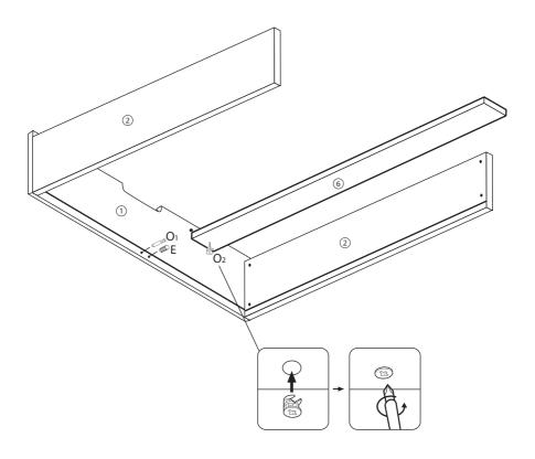
Use the wooden connectors (Part E) and bolts (Part O) to secure the underneath support (Part 6) with the front board of the drawer (Part 1).
