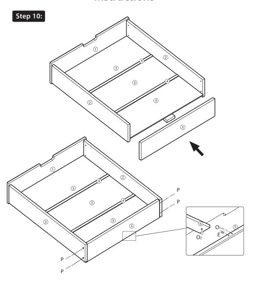
Combine the end part of the drawer (Part 5) to the assembled drawer in step 9 with screws (Part O & P) and wooden connectors (Part E)
