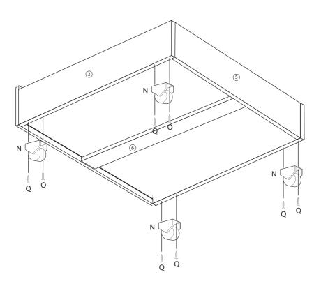
Screw the wheels (Part N) into the all corners of drawer with Part Q.
